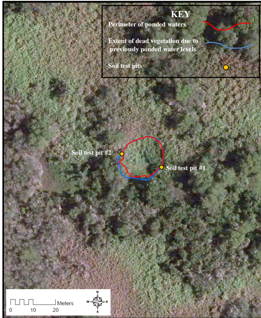
Figure 13. Mahalang Site MC1 Depicting Soil Test Pits and Perimeters of the Previously Ponded Water Line and Existing Water Line as of December 4, 2014
