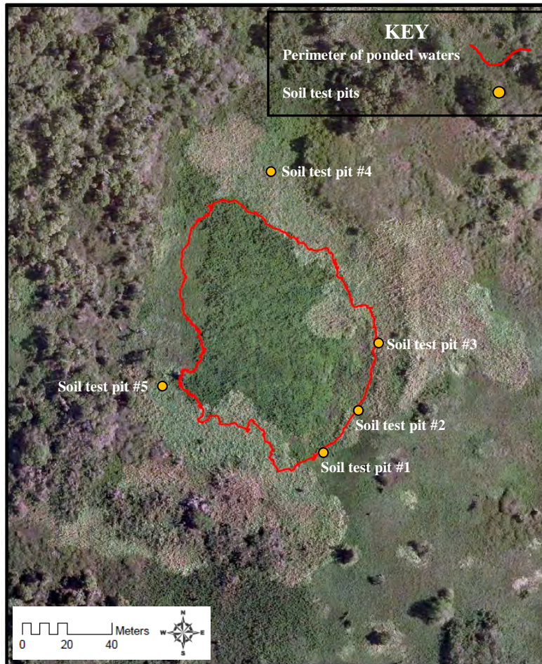
Figure 20. Bateha Site BD2 Depicting the Soil Test Pits and Perimeter of the Existing Ponded Water Line as Mapped on December 1, 2014 (Note: Data are superimposed onto an undated aerial photograph.)
