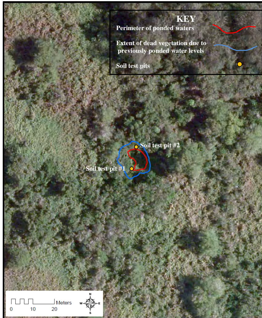
Figure 14. Mahalang Site MC2 Depicting the Soil Test Pits and Perimeters of the Previously Ponded Water Line and Existing Water Line as Mapped on December 4, 2014
