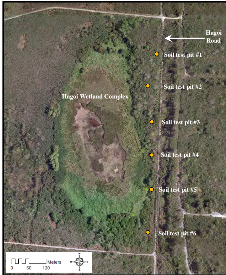
Figure 11. Hagoi Wetland Complex Depicting the Soil Test Pits adjacent to the Western Side of Hagoi Road
